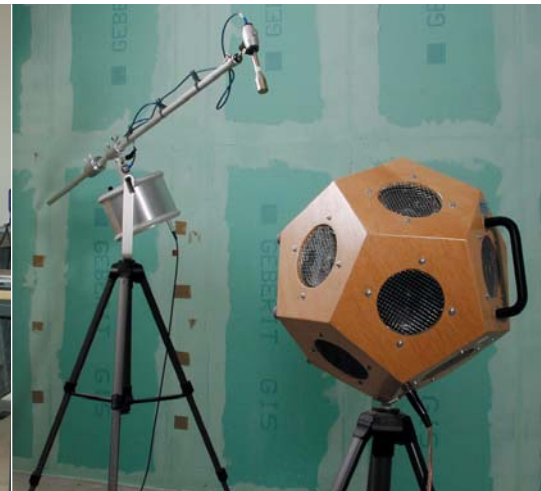
Recording and monitoring equipment set up in acoustically isolated room at Geberit's test facility.
